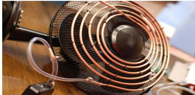
Fig. 2 Experimental setup of evaporative air conditioner
