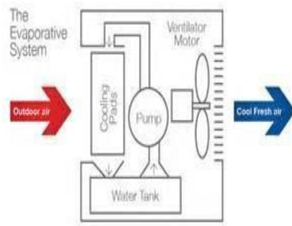
Fig.1 flow diagram of evaporative air conditioner.
