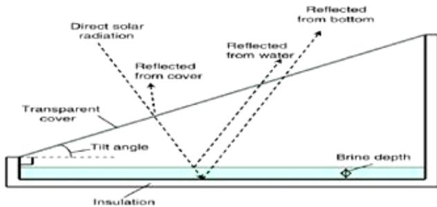
Figure 1: Schematic diagram of a basin-type solar still [1]
