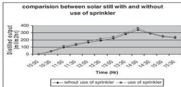
Figure 4: Use of Sprinkler in Solar Still
