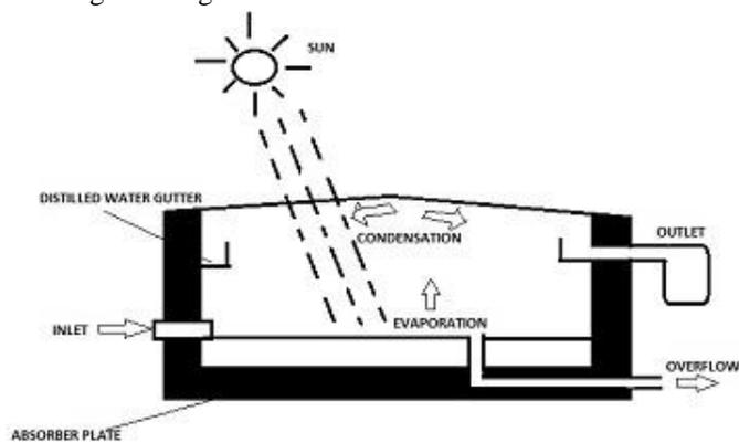
Figure 2: Basis concept of solar distillation [3]
