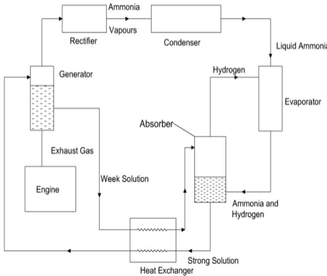
Fig 4.1 Schematic of the absorption refrigeration system using waste heat from IC engine
