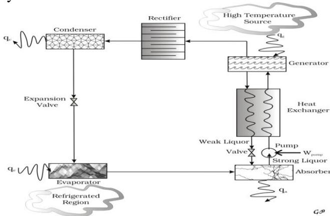
Fig. 1.3. Block diagram of Vapour absorption refrigeration system (VAR)
