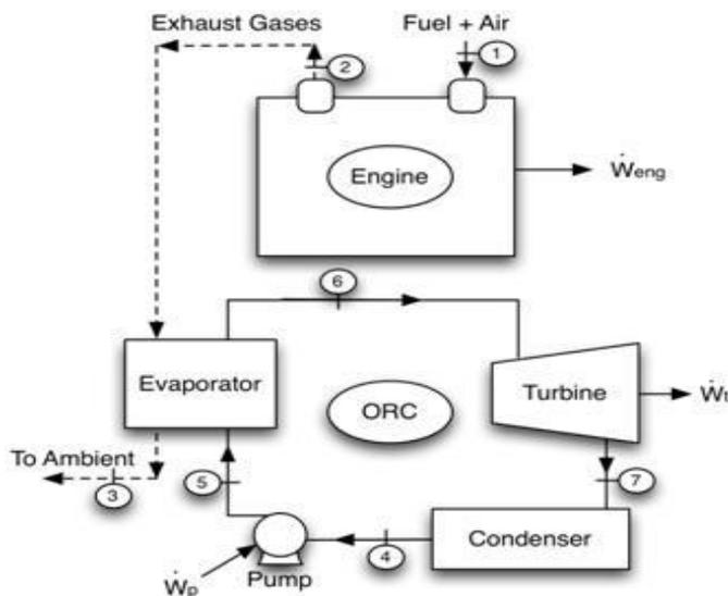
Fig. 1.1: A typical waste heat energy recovery system with ORC
