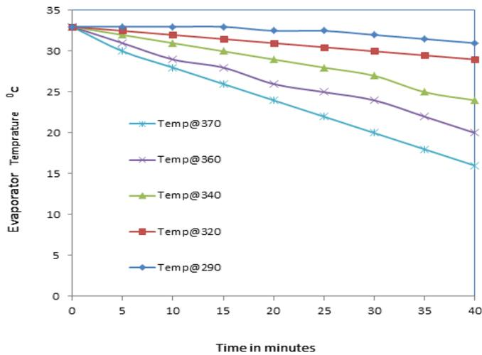
Fig 6.1: Variation of evaporator temperature with respect to exhaust temperature
