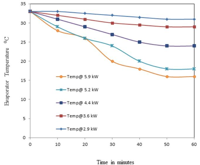
Fig 6.2: Variation of evaporator temperature with respect to brake power
