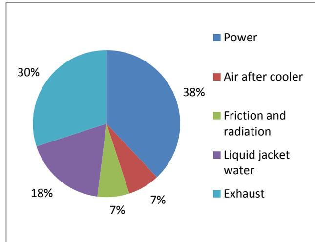
Fig. 1.2: Amounts of heat dissipated from engines
